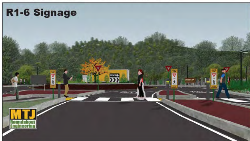
The W11-2 sign placement obstructs the view of the Yield and One Way signs
